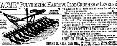
smooth the ground, white at the same time curved coulters cultivate, lift and turn the entire surface of the soil. The backward slant of the coulters prevents tearing up rubbish and reduces the draft. Made entirely of cast steel and wrought iron and therefore practically indestructible.
